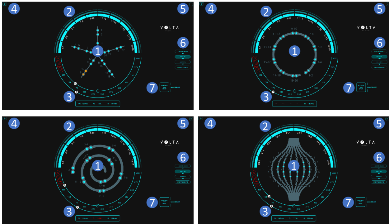
Figure 12: Pentaray (top left), Circular 20 (top right), Reflexion HD (bottom left), Orion (bottom right) Catheters VX1+ UI in analog communication mode. 1) The center of the screen displays a frame with a schematic representation of the catheter used for mapping. Catheter electrodes are numbered. If bipoles are blinking in orange / red, this indicates to the operator that the area under investigation is one exhibiting dispersed electrograms. For confirmation, the operator may stabilize the catheter in this region. 2) On the upper half-circle, 10 box sections correspond to the 10 bipoles of interest. When one or several bipole symbol(s) is / are blinking and is / are colored in orange / red, this indicates to the operator that the area under investigation is one that is confirmed as a region exhibiting dispersed electrograms. 3) The lower half-circle displays (i) the average global cycle length (GCL) as recorded by the reference catheter (R) and (ii) the average local cycle length (LCL) as recorded by the mapping catheter (M). In the lowest part of the interface, the exact values of the cycle lengths are given in milliseconds as well as the difference ratio in percentage computed as (R-M)/R . 4) Analog Procedure settings page. 5) Main menu including Logout, Help Page, About, Shutdown and Restart. 6) Procedural stages buttons: Initialization replaced by Electrograms once initialized, Mapping, Ablation, End Procedure. 7) Booster mode activation/deactivation button.
