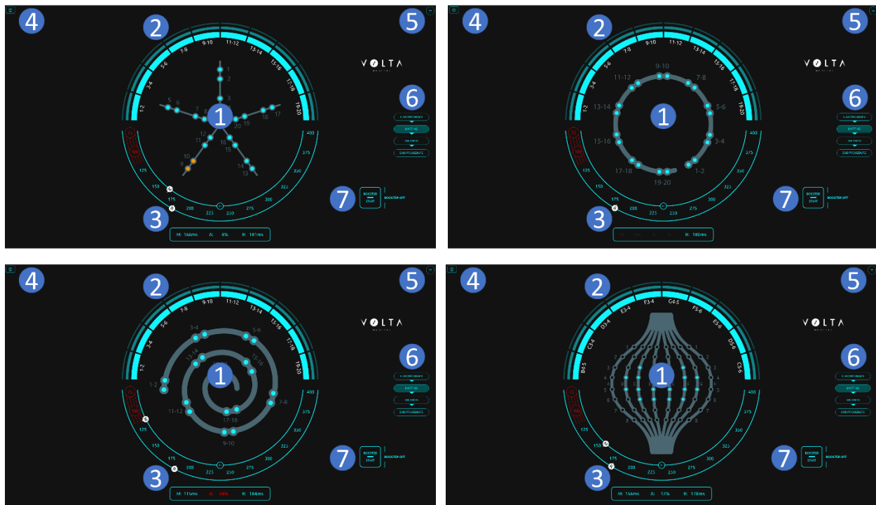
Figure 10: Pentaray (top left), Circular 20 (top right), Reflexion HD (bottom left), Orion (bottom right) Catheters VX1+ UI in analog communication mode. 1) The center of the screen displays a frame with a schematic representation of the catheter used for mapping. Catheter electrodes are numbered. If bipoles are blinking in orange / red, this indicates to the operator that the area under investigation is one exhibiting dispersed electrograms. For confirmation, the operator may stabilize the catheter in this region. 2) On the upper half-circle, 10 box sections correspond to the 10 bipoles of interest. When one or several bipole symbol(s) is / are blinking and is / are colored in orange / red, this indicates to the operator that the area under investigation is one that is confirmed as a region exhibiting dispersed electrograms. 3) The lower half-circle displays (i) the average global cycle length (GCL) as recorded by the reference catheter (R) and (ii) the average local cycle length (LCL) as recorded by the mapping catheter (M). In the lowest part of the interface, the exact values of the cycle lengths are given in milliseconds as well as the difference ratio in percentage computed as (R-M)/R . 4) Analog Procedure settings page. 5) Main menu including Logout, Help Page, About, Shutdown and Restart. 6) Procedural stages buttons: Initialization replaced by Electrograms once initialized, Mapping, Ablation, End Procedure. 7) Booster mode activation/deactivation button.
